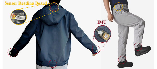
Figure 4. Prototype of our full-body garment-based motion capture system. The loose-wear jacket and pants are embedded with six IMU sensors and two central circuit boards for data acquisition in total.
