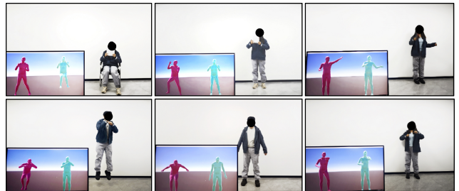
Figure 1. Garment Inertial Denoiser (GIP) can denoise real-time loose wearing IMU data, enabling robust full-body motion capture.
